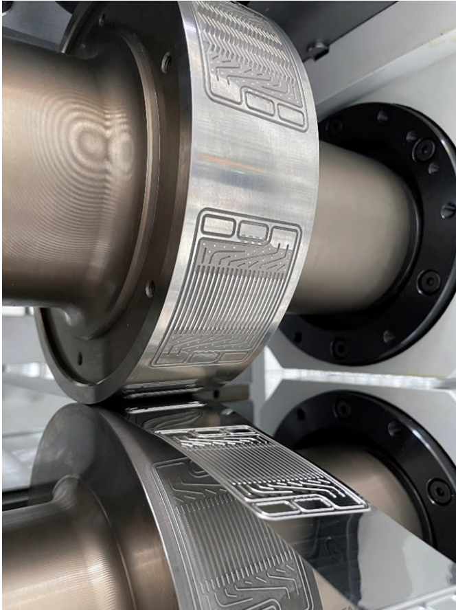
Fig. 1 Roll embossing of bipolar plates using BPPflexRoll. In the newly developed technology, the structure of the bipolar plate is embossed by a pair of rollers.
